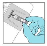
3. Unwrap an individual MiOXSYS Sensor and place into MiOXSYS Analyzer.
