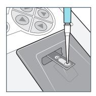
Using a pipette, transfer 30µL of sample to the Sample Application Port of the inserted MiOXSYS Sensor.
